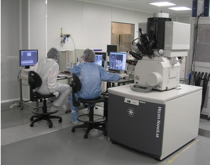
In the Clean Room facilities of the INA-LMA, several lithography facilities permit to pattern structures at the micro- and nano-meter scale and to create devices. In particular, the two dual beam instruments (Helios 600 and Helios 650) assigned to the nanolithography and lamellae preparation areas are located on two concrete platforms inside the 125 m<sup>2</sup> 10,000-class Clean Room.
