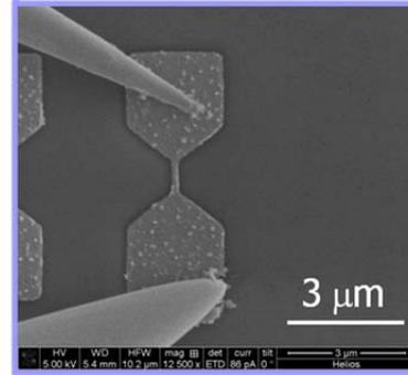
Lamellae preparation (Omniprobe<sup>®</sup> micromanipulator)
