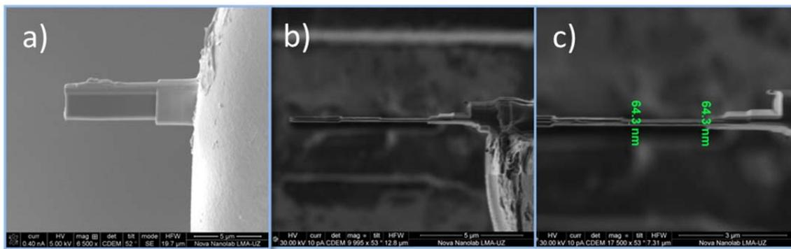
a) Electron image of lamella of organic magnetic tunnel junctions on the grid. b) Final view of the lamella, ion image c) details and thickness of lamella by ion image, the final process was made at low temperatures (-160 °C)
