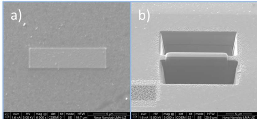
a) Pt deposited by e- over multilayer organic magnetic tunnel junctions b) View of milling by i+ beam during the process to make lamella previous to the lift out.
