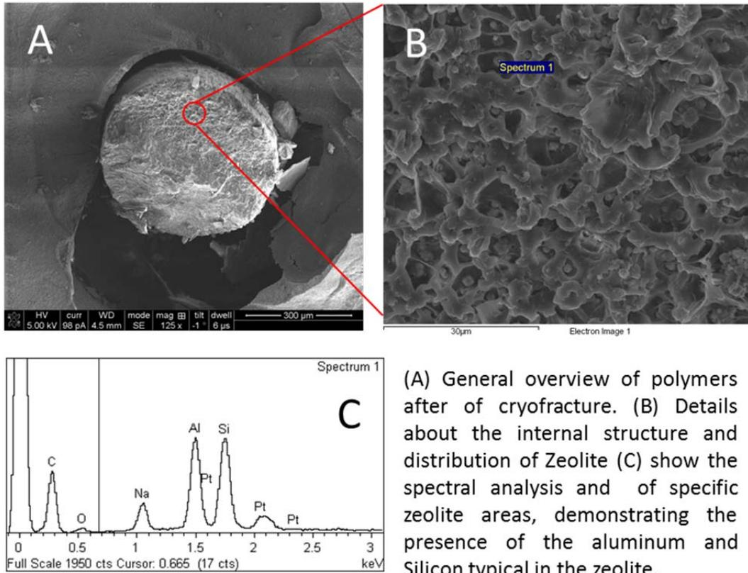
(A) General overview of polymers after of cryofracture. (B) Details about the internal structure and distribution of Zeolite (C) show the spectral analysis and of specific zeolite areas, demonstrating the presence of the aluminum and Silicon typical in the zeolite.
