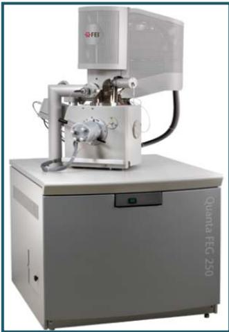
The FEG column in Quanta 250 allows beam deceleration, which permits to achieve a resolution of 1.4 nm even at 1 kV electron landing voltage. The Quanta equipment can work under three different pressure ranges, the maximum pressure being 2600 Pa. This permits observation of life-sciences samples without previous metallic coating, i.e., studies in environmental conditions (ESEM).
