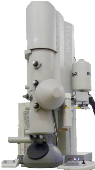
The Tecnai F30 (FEI company) is a versatile high resolution Transmission Electron Microscope. It can work in TEM or STEM (Scanning-Transmission) modes. It is equipped with all the analytical techniques to obtain morphology, structure and composition information with atomic resolution.
