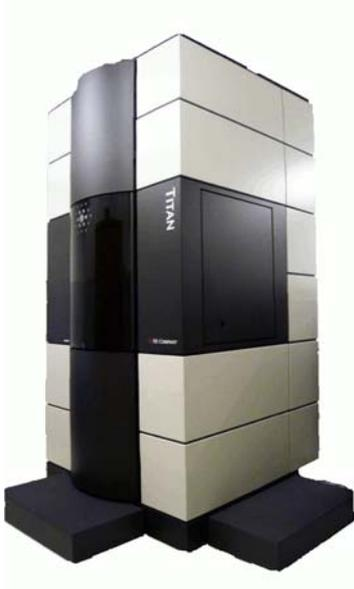
The Titan High-Base has a spherical aberration corrector (CEOS Company) at the objective lens, the lens that forms the image. It is therefore the ideal instrument for ultra-high resolution imaging (HRTEM). This microscope also has a biprism for Electron Holography analysis and a Lorentz Lens to perform High Resolution Lorentz Microscopy.
