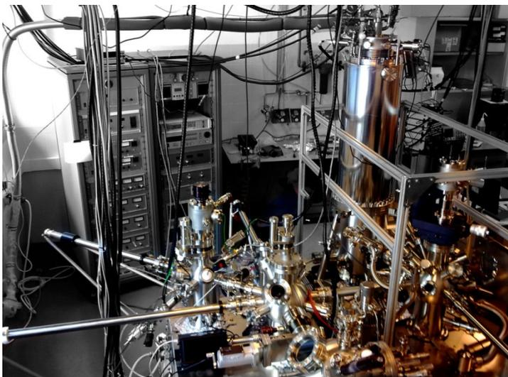
This equipment is specifically oriented to investigate atomic scale magnetism and to high resolution spectroscopy (0.1 meV) of molecules and atoms, as well as to study the physical-chemical phenomena of surfaces function of temperature and gas dosing.
