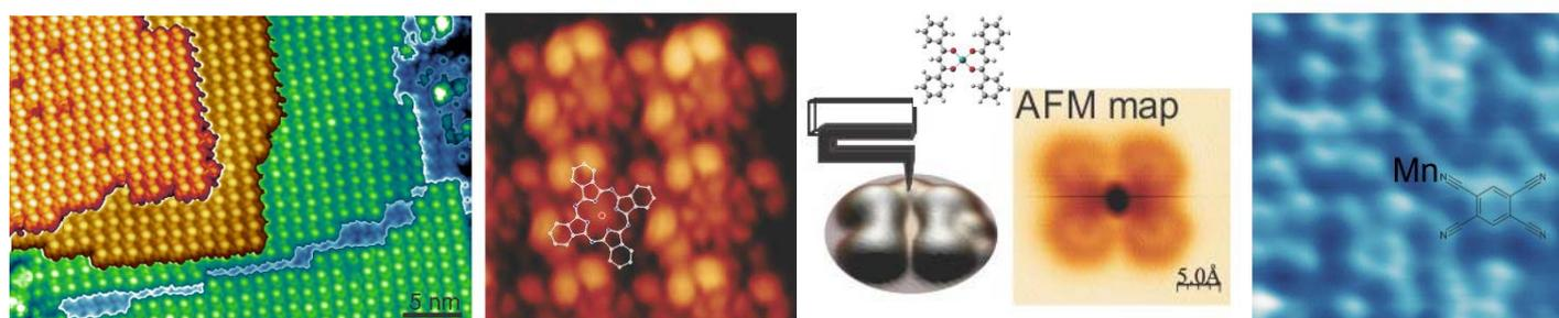
Caption: From left to right. STM topography of a 3 layer thick  $\pi$ -stacked FePc film. Zoom into one of the layers. STM topography and simultaneous force map of a Ruthenium based complex. Atomically resolved force map of a Mn-Tetracyanobenzene coordinated network.
