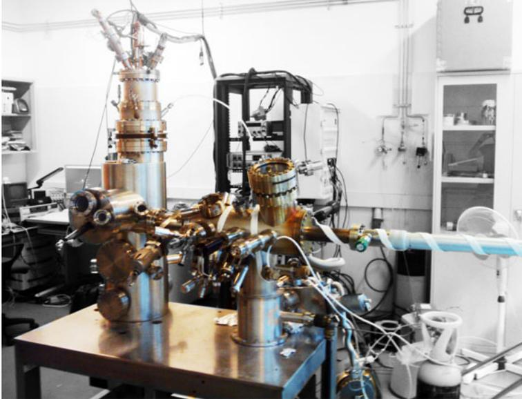
This equipment is devoted to investigate metal-on-metal epitaxy of rare earths. It is specially oriented to the growth of magnetic thin films and nanostructures.
