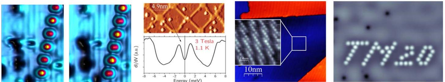
Caption: From left to right. Binary information encoded in single Co atoms with up/down spin represented by yellow/red colors. The same chain with contrast reversed. Example of energy resolution in quantum spectra (Co atoms over  $\text{Cu}_2\text{N}$  monolayer).  $\text{Ni}_3\text{C}_4$  over a Ni (111) surface stabilized by a partial pressure of  $10^{-6}$  mbar propene at 500 °C. Example of atomic manipulation to build the logo of 'Tercer Milenio 20' using 44 atoms.
