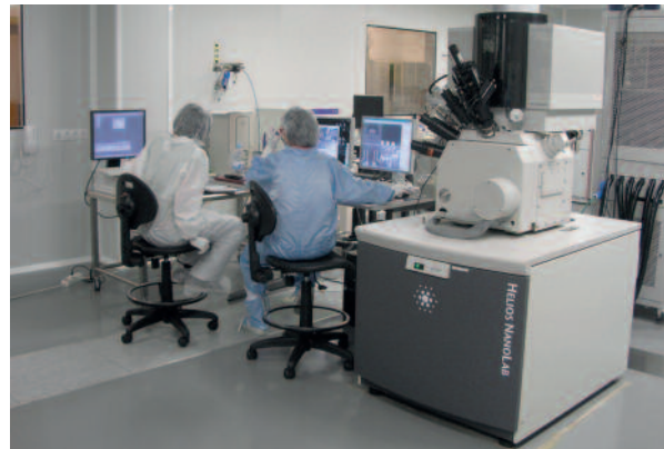
Helios 600 dual beam equipment installed inside the Clean Room of the INA building.
