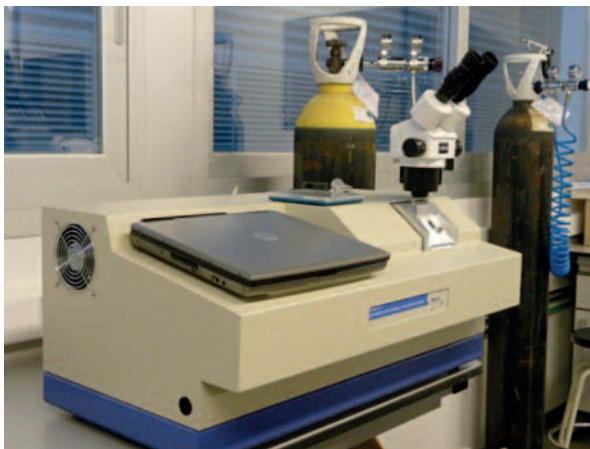
Ion mill equipment to obtain electron transparent areas in the samples for the TEM observation.
