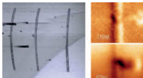
Overview of three Py nanowires with different curvature. On the right side the magnetic signal before and after nucleating a DW at the trap upon application of 2 Tesla perpendicular to the wire is shown (4.2 Kelvin).
