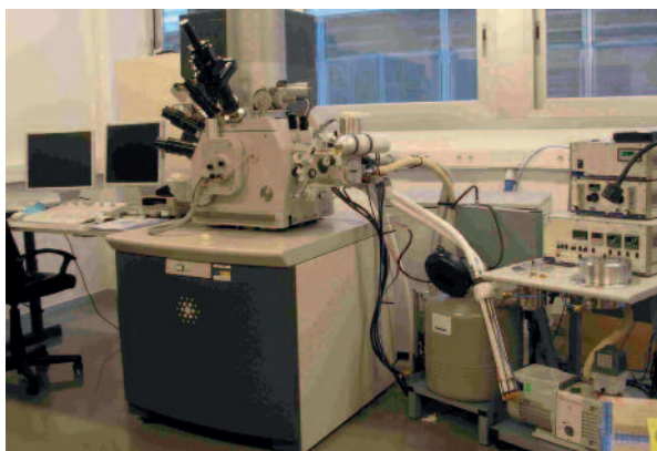
Nova 200 dual beam equipment and the cryo-transfer setup, installed at INA building
